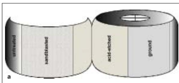
**Fig 1** (a) Model of a surface modified abutment with 4 different surface treatments—standard machined titanium, sandblasted ( $\text{Al}_2\text{O}_3$ ), acid-etched (hydrofluoric acid), and ground. (b) Modified abutments in situ.
